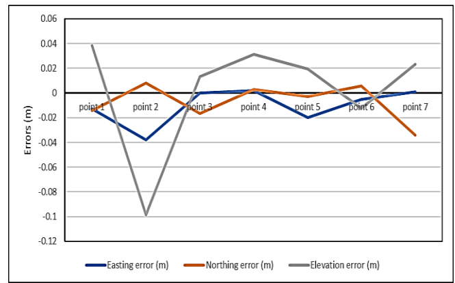
Fig. 17: ICPs Errors for DG/reference aligning technique
